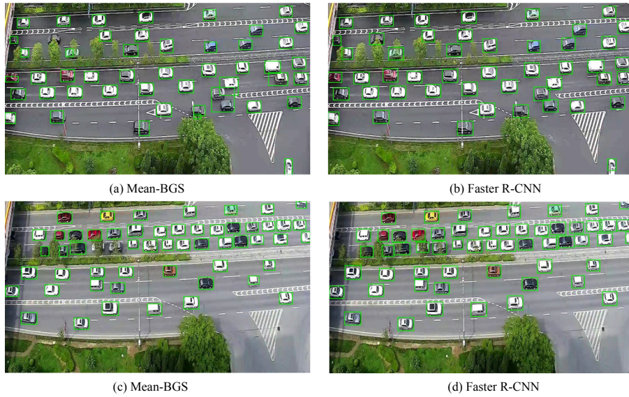
Fig. 5. Detection results in Scenario I on the collected DNVD dataset: daytime vehicle detection. Top: normal traffic, Bottom: congested traffic.
