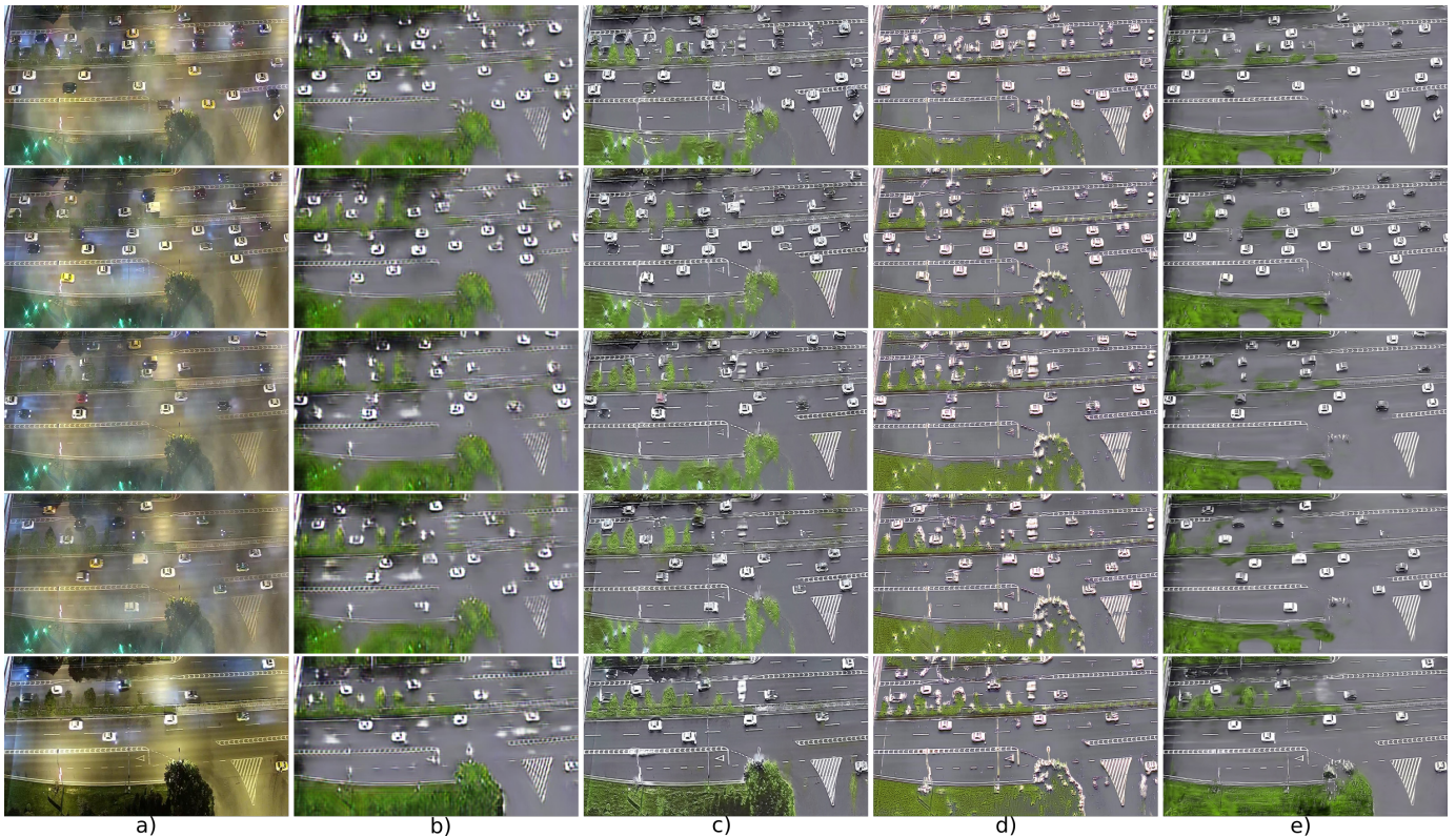
Figure 8: Visualization results of image translation from nighttime to daytime. a) is target nighttime image, b) to e) are the image translation results of UNIT n2d [12], CycleGAN n2d [11], GcGAN n2d [46], and proposed method, respectively.
